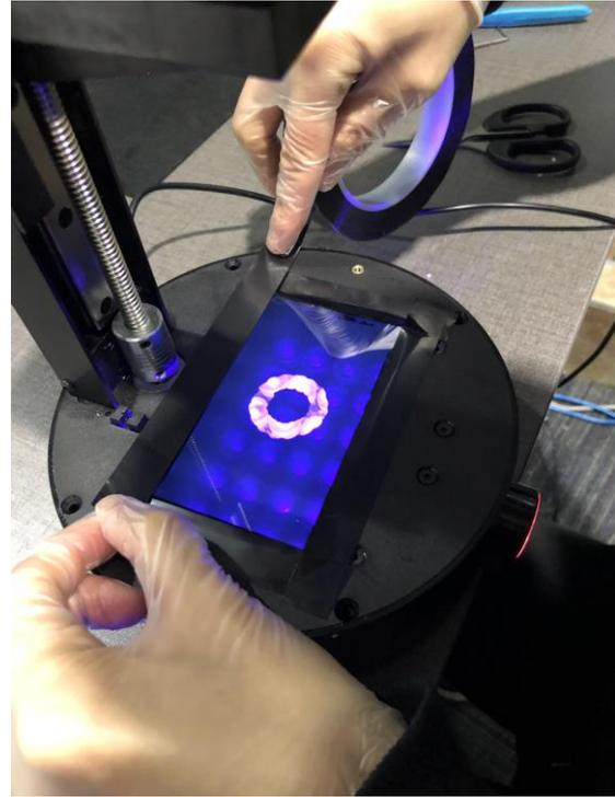
5. Tighten the two screws of the resin tank and install it.
