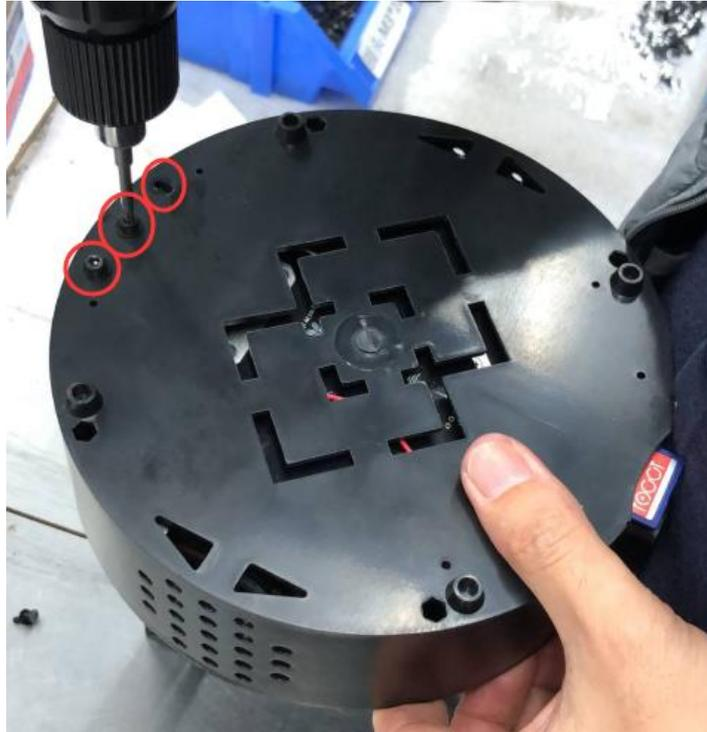
2. Remove the resin tank and loosen six screws on the panel top (remember to collecting the falling nuts).
