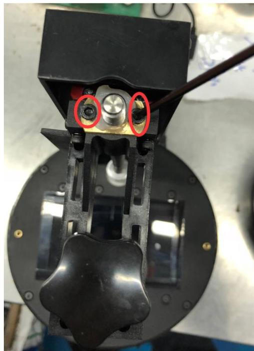
3. Push the copper nut into the guide rail.
