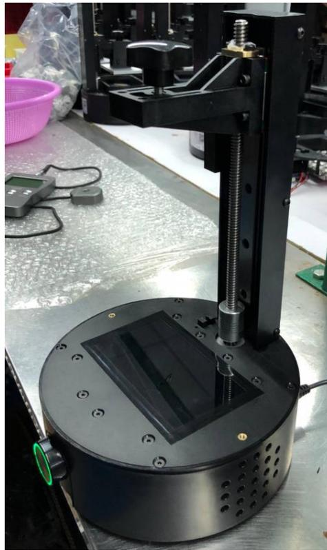
2. Loosen the copper nut mounting screw.
